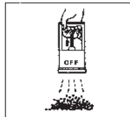
Magnet turned OFF Releases by Piling Up Lever.
